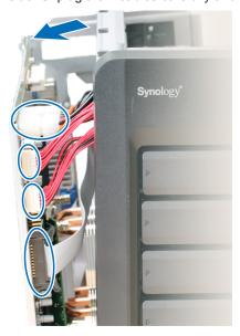
**d** Lay down the inner panel with the 2 cables still connected to its bottom. If you need more space when installing your memory module, you can choose to unplug them.
