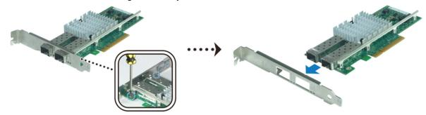
2 Replace the long bracket with the short one, and tighten the 2 screws to secure the short bracket.
