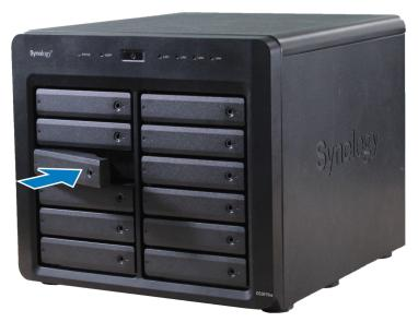
2 Pull the hard drive tray handle in the direction as indicated below to remove the hard drive tray.
