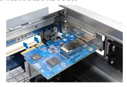
d Push back the tab to secure the newly inserted card.
