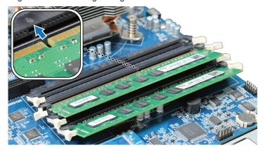
**c** Push down on the memory module with firm and even pressure. The retaining clips will snap into position as the module is correctly inserted.
