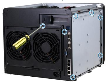
**Note:** When you remove the case, you expose sensitive internal components. Avoid touching anything other than the memory assembly when you remove or add memory.
