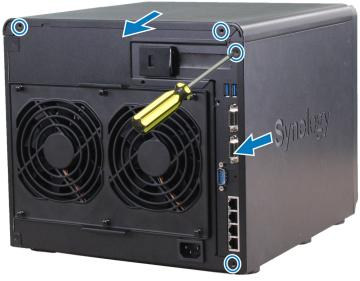
**b** Remove the 7 screws that secure the inner panel.
