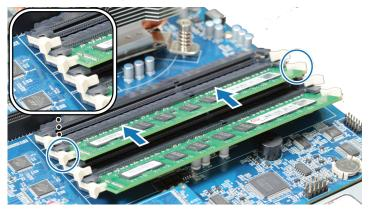
**Note:** Hold the memory module by its edges, and do not touch the gold connectors.
