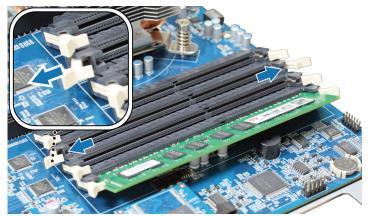
**b** Align the notch on the gold edge of the module with the notch in the memory slot.
